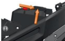
④ Press the discharge plug locker and disconnect the discharge plug.
