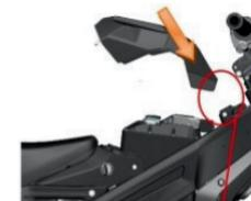
③ Well fit battery fixing device dropout on the pins.
