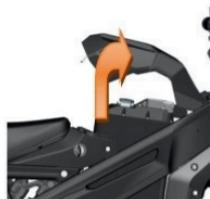
② Rotate the battery case cover clockwise.
