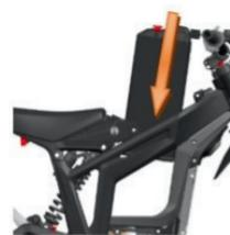
① Install the battery into the holder.
