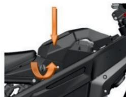
① Press the battery case cover and turn the key counterclockwise to unlock the battery case cover simultaneously.
